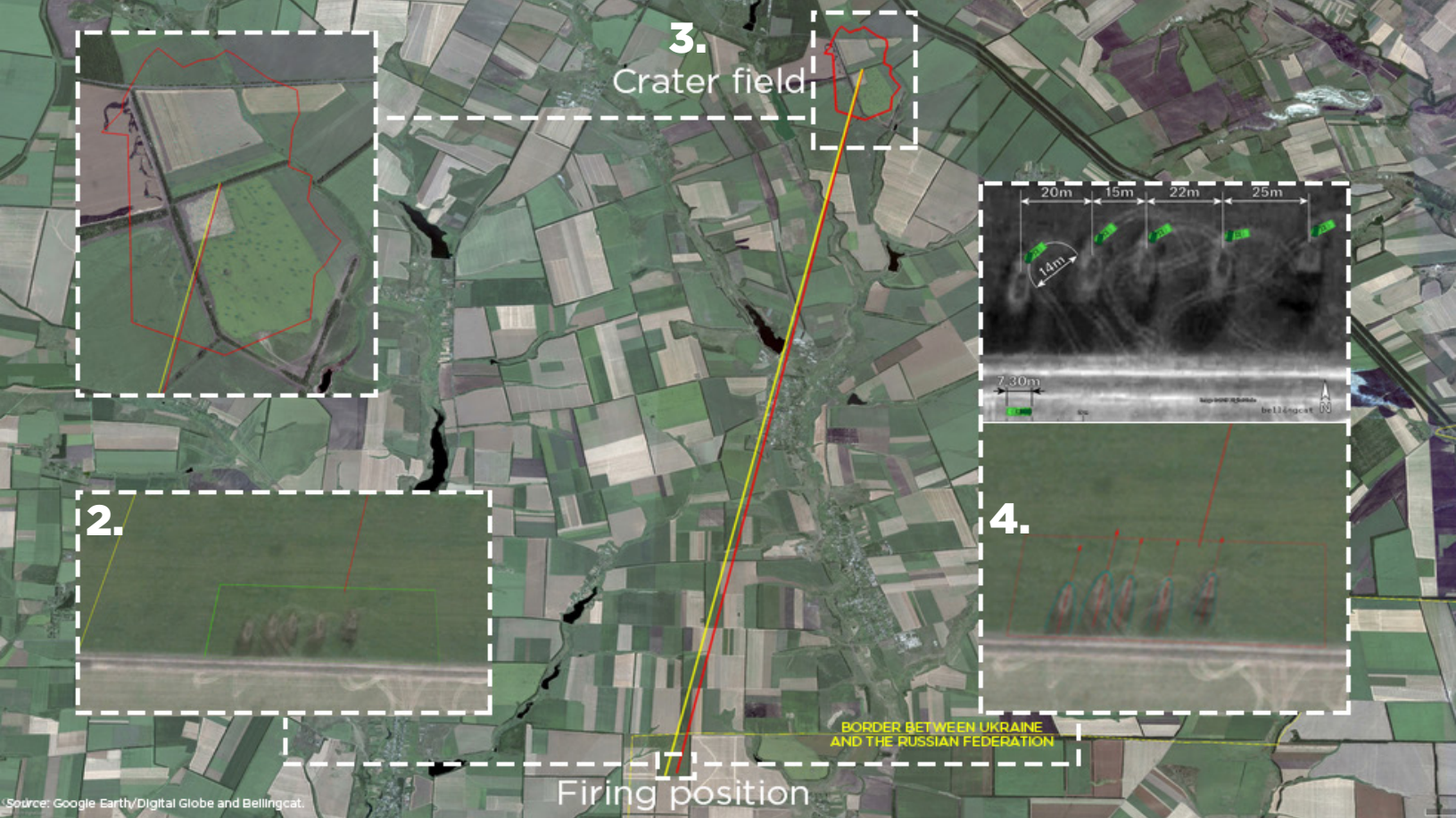
Maps showing the average trajectory of craters measured at the Amvrosiivka impact site, the approximate direction of fire indicated by burn marks on the ground near Seleznev, and the position and size of multiple rocket launchers used during the attack based on the position of track marks at the launch site. Source: Satellite image from Google Earth/Digital Globe.
